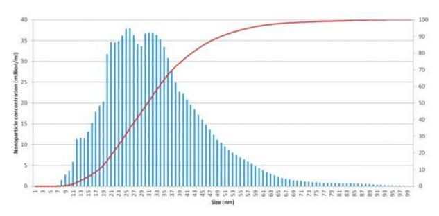
Size distribution of colloidal silver determined using nanoparticle tracking analysis (Nanosight NTA 2.2). The concentration at each size category (nm) in shown as 106 particles/ml. Cumulative percentage undersize is shown in red (%).
